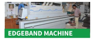
To add on elegance to the finished doors, the edges are banded using the edge band machine to secure the edges of the doors. This machine also trims edges and ensures a complete processing option and marvelous finishing.
