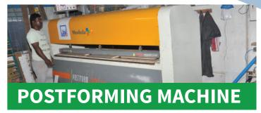
Adding Lamination to the curved edge doors is manually not possible. So, we use the imported post forming machine to attain perfect finish for post forming doors and full round tops.
